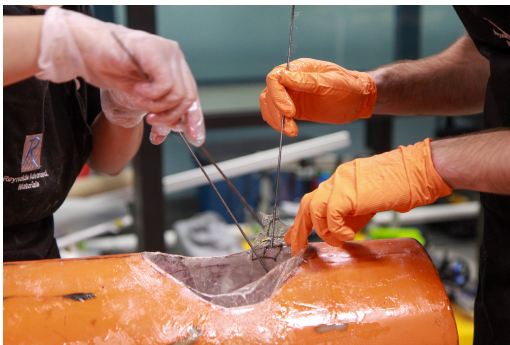
Figure 4: Using welding rods to place strips.
