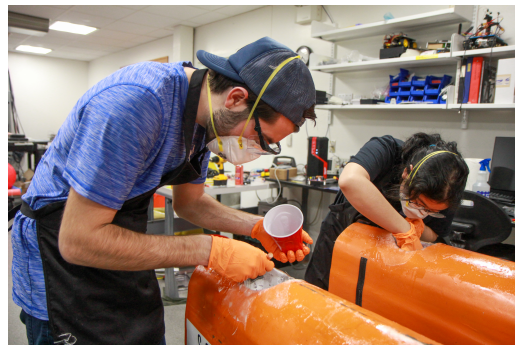
Figure 5: Painting on epoxy onto fiberglass.
